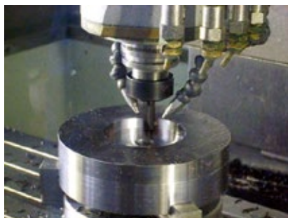
Carbide End Mills Ø10mm, z=4, steel 34CrNiMo6 (30 HRC), Coolant: Air; Minimum lubrication - Tested tools: 2x4 Source: Carmex, Maalot, ISR
